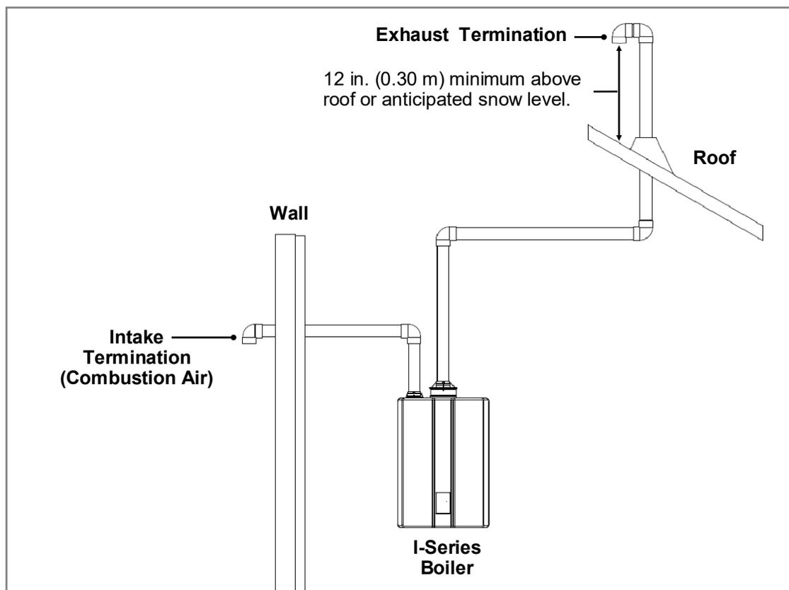
Fig 1. New I-Series Boiler Venting Configuration (Example 1)
