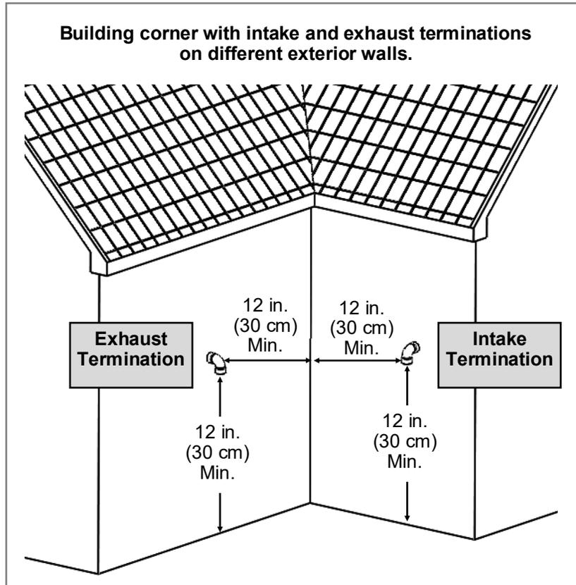
Fig 2. New I-Series Boiler Venting Configuration (Example 2)
